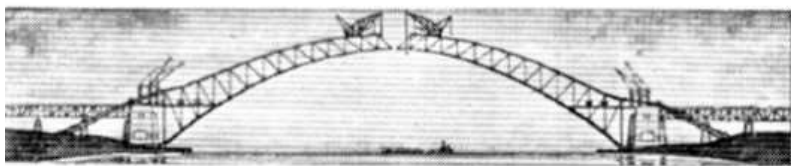
(d) Arch almost completed; gap being closed by easing out ropes one by one on both sides
