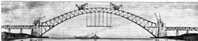
(e) Gap closed; arch finished; deck hangers and deck erected as cranes retreat along top chord
